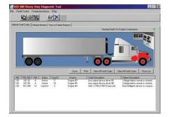
The MD-300 is the only diagnostic software on the market that includes a Graphic Vehicle Interface (GVI) that **visually** displays what components are reporting fault codes. Red indicates an active fault code, yellow indicates an inactive fault code, and green indicates no fault codes. You can instantly determine if a failure is affecting more than one system on the vehicle!
