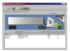
Based on these fault codes, MD Tools patented search technology filters out hundreds of unnecessary parameters, allowing the technicians to choose from only those parameters that correspond to the affected component for quicker diagnosis. For more complicated problems, technicians can view 15 parameters at once.
