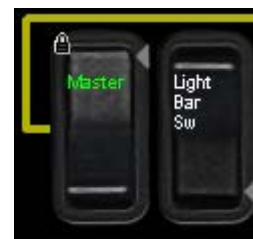
Switch shown in the on position with lock
