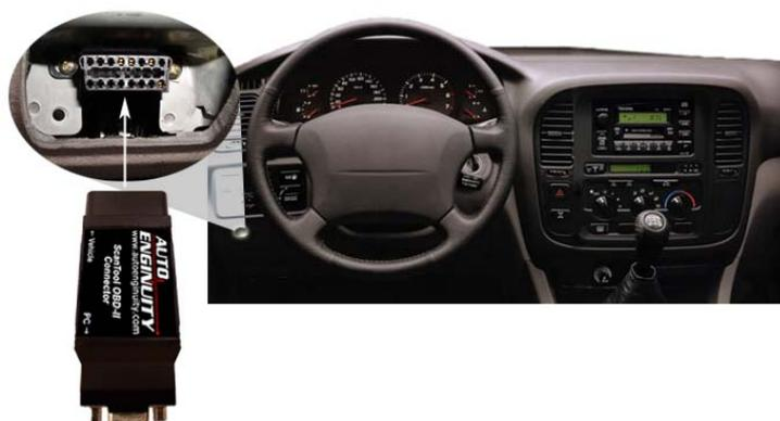
The DLC is usually exposed and accessible without a tool. (Notable exceptions being BMW which requires a flat-head screwdriver to remove a plastic cover, and Mercedes and MINI which hides the DLC under a cover.) Exceptions to the standard location include the ashtray/console area, or in the rear seat. If you have trouble finding the DLC, see *Appendix A* or consult your vehicle's Owner's Manual for more details. Once you locate the DLC, plug
