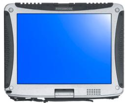
Panasonic Toughbook: CF-19 Fully ruggedized computer. Designed using MIL-STD-810f test procedures. Full magnesium alloy case, vibration and drop-shock resistant, built in carry handle, removable shock mounted hard drive, moisture and dust resistant design. Converts into a tablet computer. 10.4" touch or digitize monitor.
