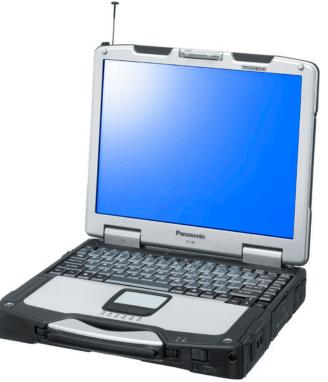
Panasonic Toughbook: CF-30 Fully ruggedized computer. Designed using MIL-STD-810f test procedures. Full magnesium alloy case, vibration and drop-shock resistant, built in carry handle, removable shock mounted hard drive, moisture and dust resistant design. 13.3" monitor that is available with touch screen options.
